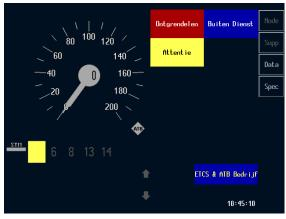
Figure 3. DMI ETCS in SLT trains during ERTMS pilot. Left: ETCS level 2. Right: STM ATB.
